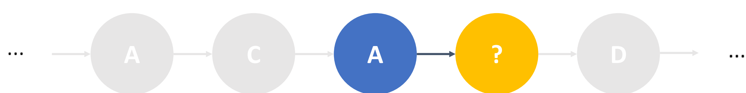
Figure 1 In a first order Markov chain, the current value predicts the next value.
